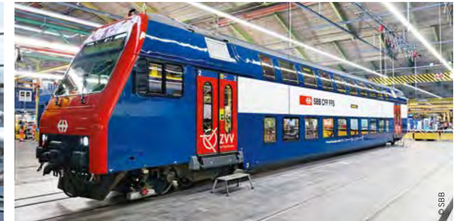
The first modernized driving cab Bt DPZ of a double-decker commuter train for the S-Bahn Zurich with air-conditioned passenger cars
