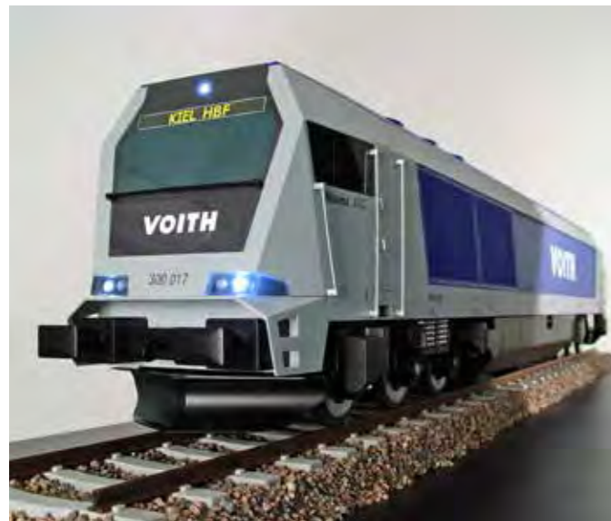
Co-development of the largest diesel-hydraulic locomotive in the world with a power output of 3600 kW
