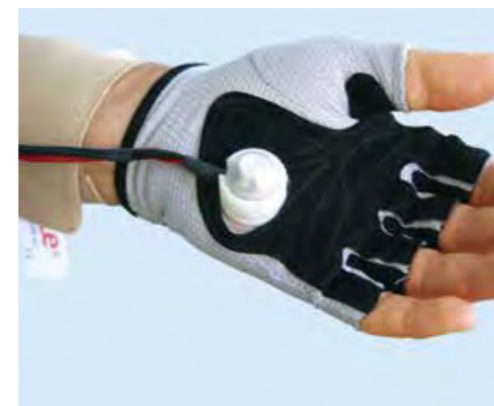
Development of a vibrotactile stimulator used to treat pain sufferers in Coordinated Reset® therapy
