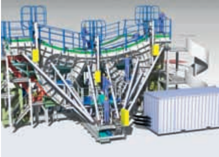
Injection-molding machine for the manufacture of cement elements for support structures in thermal solar power plants
