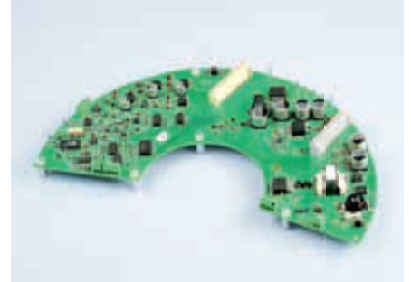
Electronic measuring equipment with lock-in technology for absorption photometry
