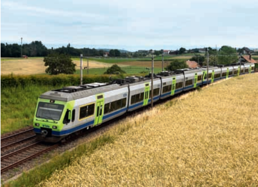
Low-floor railcar train set Type NINA of the BLS for urban passenger transport
