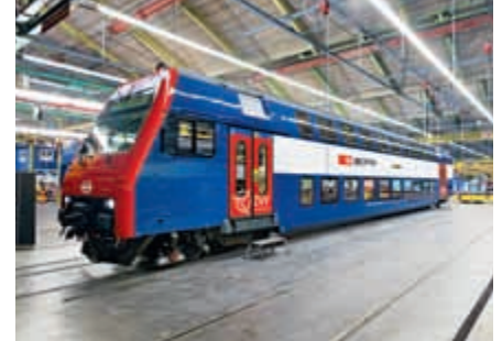
The first modified control car Bt DPZ of a double-decker commuter train of the S-Bahn Zurich with air-conditioned passenger compartments
