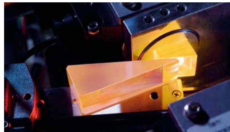
Optical Elements for FT-NIR-Spectrometers (Fourier Transform Near Infrared)
