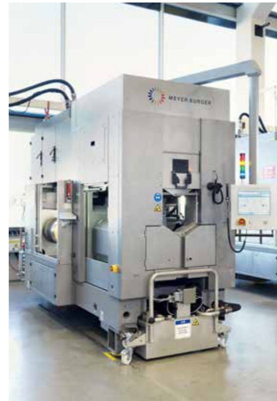
Diamond wire saw for the slicing of monocrystalline wafers
