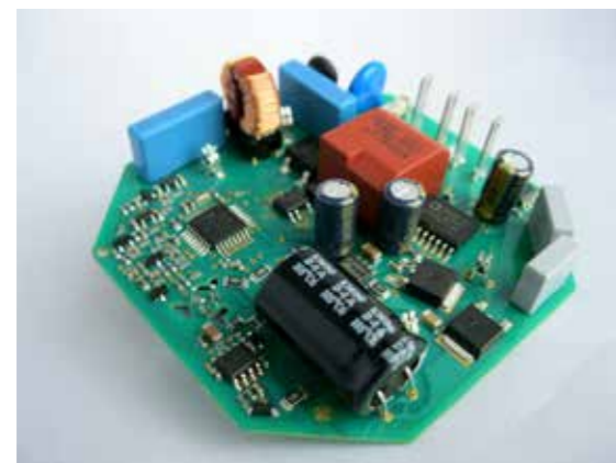
Power PCB for 230V fan with MOD-BUS Interface
